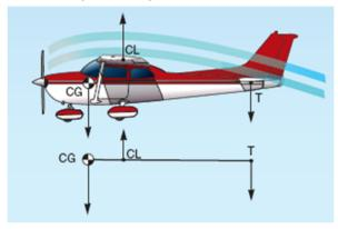
This design causes a natural tendency for the airplane to nose down, reducing the angle of attack. To counteract this, the horizontal stabilizer and elevator surfaces of an airplane are designed to produce a downward force, which 'holds up' the heavier nose area by pivoting the airplane around the Center of Lift. When an airplane stalls, if the elevator pressure is relaxed, the Center of Gravity will fall naturally.
