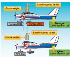
wing, requiring it to produce slightly more lift to compensate. Also, because any airfoil that produces lift also produces drag, the amount of drag caused by the horizontal stabilizer depends on the force it must produce.
