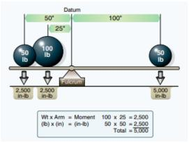
CG - Once all individual weights in an aircraft are considered, the *Center of Gravity* (CG) represents a sort of 'average position' of the weights. When balancing an object by a fingertip, objects balance on their center of gravity. When computing weight and balance for airplanes, the position of the CG is assumed to be some distance from the datum, represented as an *arm*, or *inches aft of datum*.
