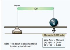
• **Arm** - The *distance* from the datum. The further that an object is from the datum, the longer the arm. Arm is usually expressed as *inches aft of datum* (positive arm numbers) or *inches forward of datum* (negative arm numbers). **This is also sometimes called a** *station in some POHs.*
