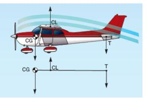
To counteract this, the horizontal stabilizer and elevator surfaces of an airplane are designed to produce a *downward* force, which 'holds up' the heavier nose area by pivoting the airplane around the Center of Lift. When an airplane stalls, if the elevator pressure is relaxed, the Center of Gravity will fall naturally.
